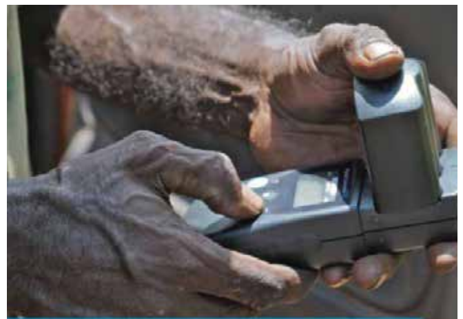
Sampling water at a public tap to check the chlorine levels of water delivered to customers.
