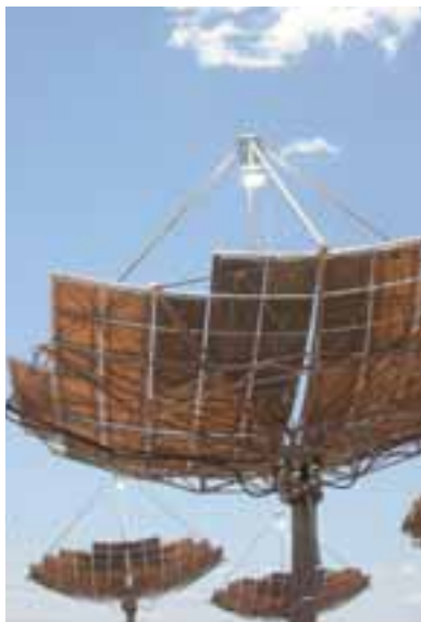
ABOVE ► SOLAR DISH CONCENTRATORS IN CENTRAL AUSTRALIA
